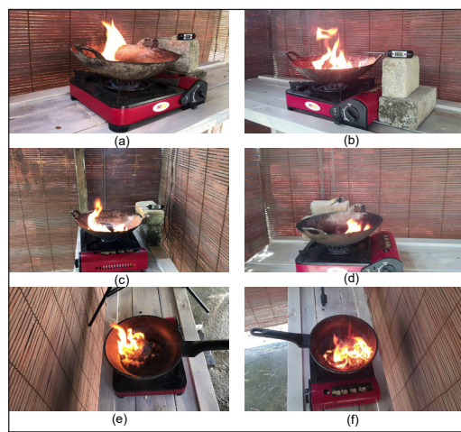
Figure 3. A sample of six images represent six different positions of pan fire object from red, green, and blue (RGB) dataset: (a) 50 cm and 45° left, (b) 50 cm and 45° right, (c) 50 cm and side right, (d) 50 cm and center, (e) 75 cm and top left, and (f) 75 cm and top right, respectively
